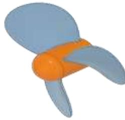
**Fig. 1 CAD Model of Propeller**
