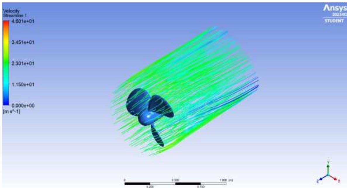
*Fig. 8 Nickel-Aluminium-Bronze Velocity Gradient.*
