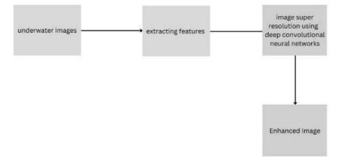
*System Design*: The system architecture shows the underwater image enhancement in two steps. First our system takes an underwater image as input, then it will identify the color co- relation in every pixels, then it will remove the fogging using the image processing techniques. In second step our system will apply Deep Learning Algorithm to enhance the underwater image without any data loss and noise.
