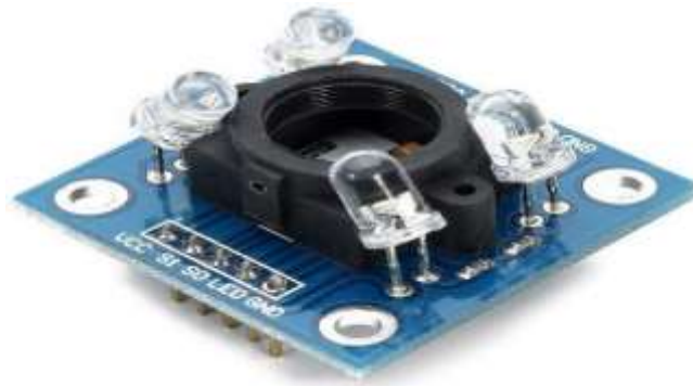
Fig. 4. Tcs3200 to extract colour from leaves .
