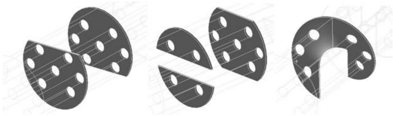
Figure 2 : Types of baffles (a) Segmental baffles, (b) Double segmental baffles, (c) Helical baffles
