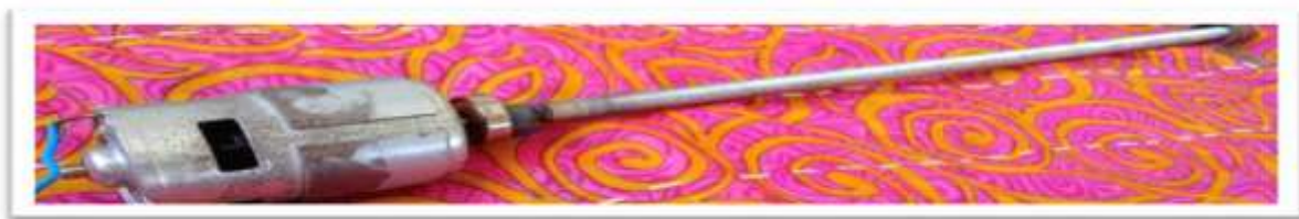
Fig. 1 - Lead screw mechanism
