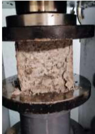
Fig. Split Tensile Test of Cube
