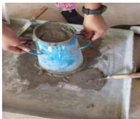
Fig 6.1: Slump cone test
