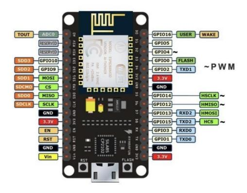
There is a candid difference between Vin and VU where former is the regulated voltage that may stand somewhere between 7 to 12 V while later is the
