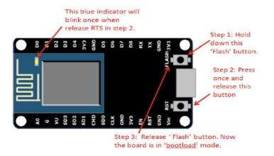
The interface of the module is mainly divided into two parts including both Firmware and Hardware where former runs on the ESP8266 Wi-Fi SoC and later is based on the ESP-12 module. The firmware is based on Lua – A scripting language that is easy to learn, giving a simple programming environment layered with a fast scripting language that connects you with a well-known developer community.
