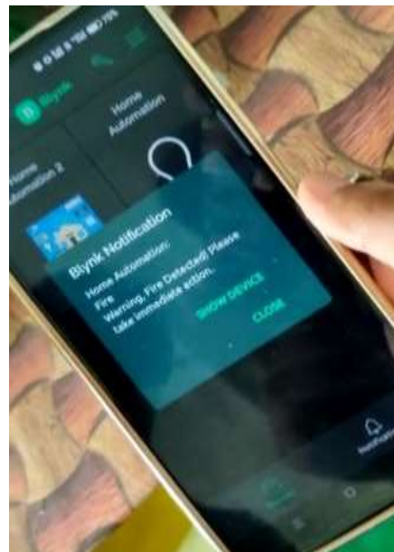
Fig. 7. Receiving fire notification
