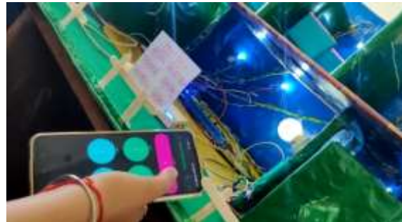
Fig. 5. Switching the LEDs using Blynk (Status: ON)
