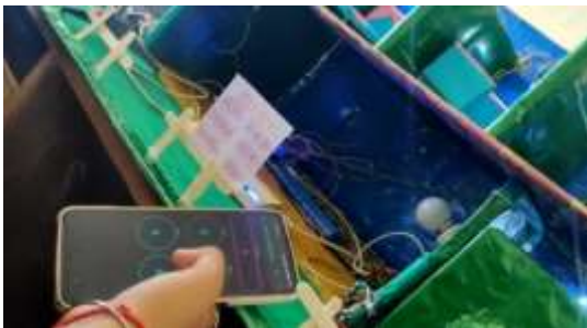
Fig. 4. Switching the LEDs using Blynk (Status: OFF)
