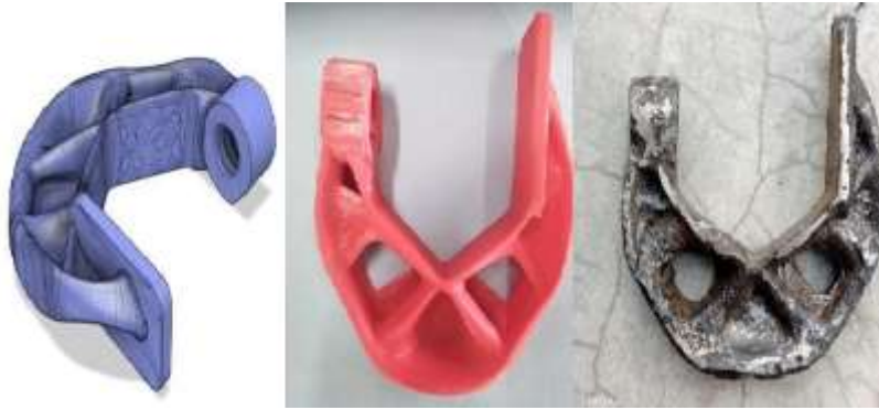
Fig.2.Generative Design Model,PLA Model and Casted Model
