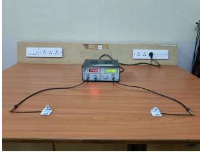
Fig. 5 Folded state antenna testing
