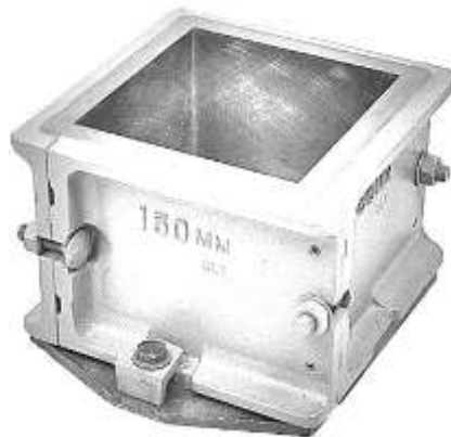
Figure 1. ISI approved CI Concrete Cube Mold of size 150 x 150 x 150mm with base plate.
