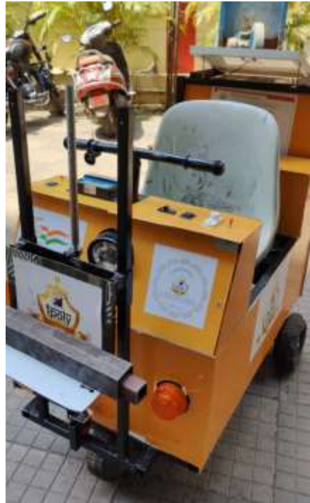
Fig 2 : Final Model of Forklift
