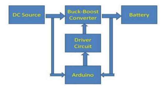
Solar PV panels are used to generate the electricity this generated DC voltage is given to the Buck-boost converter circuit. Buck-boost converters are a form of switching-mode power supply that can supply a regulated DC output from a source voltage either above or below the desired output voltage. The Arduino is the controller circuit, It is control the whole circuit.
