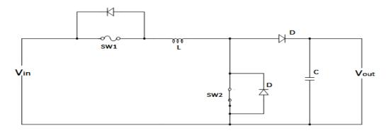
At boost mode SW2 is closed and SW1 is always Close. Because the buck mode is always on in the circuit. The Boost mode is on when the input voltage is lesser or lower than 14v. In this mode the voltages is steped up. At boost mode when we supply input to 9v then the converter is convert or steped up the voltage and give output 14v for battery Charging.
