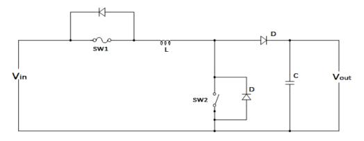
At buck mode SW1 is closed and SW2 is open. The buck mode is on when the input voltage is greater or higher than 14v.In this mode the voltages is steped Down. At buck mode when we supply input to 18v then the converter is convert or steped the voltage and give output 14v for battery Charging.
