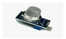
The MQ 135 sensor is a signal output indicator instruction. It has two outputs analog output and TTL output The TTL output is low signal light that can be accessed through the IO ports on the Microcontroller. This Temperature, presure Sensor is an integrated environmental sensor which is very small-sized with low power consumption.
