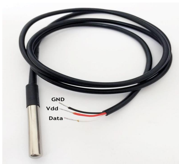
Figure 4: The Diagram of DS18B20 Temperature Sensor.
