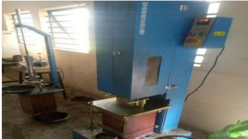
Figure1: Manual and Mechanical Marshal Compactor
