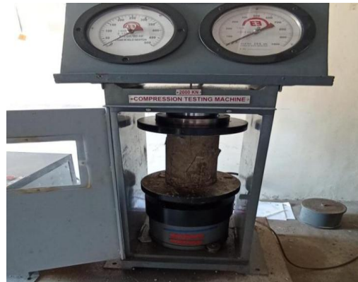
Fig 2 : Compressive strength test on cylinders
