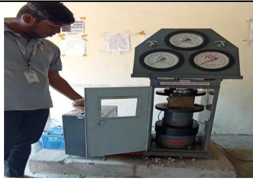
Fig 1 : Compressive strength test on cubes
