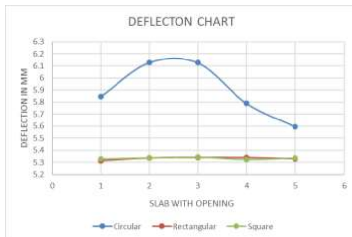
FIG.4.19. DEFLECTION VARIATION DIAGRAM WITH OPENING SHAPES
