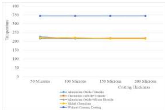
Fig 26. Comparison of temperature distribution of Ceramic coated piston with uncoated piston.
