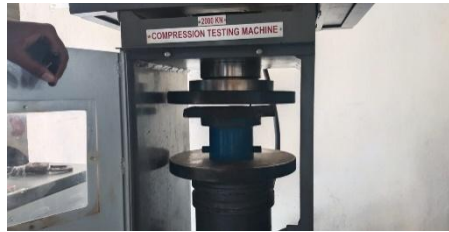
Fig 2 : Compression test of tiles
