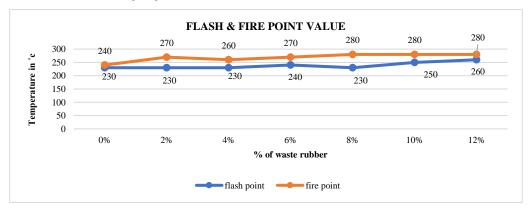
**Description of Flash and Fire Point Test:** The IS specifications for the Flash point of penetration grade of 80/100 bitumen is minimum of 225° c (>225 ° c). The flash point values are obtained as per the specifications. Hence, the mixing of waste rubber in bitumen doesn't decrease the flash point property.
