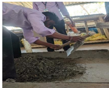
Fig. 5.7 Mixing of Cement mortar with coir
