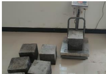
Fig. 7.5 weighing of test specimens
