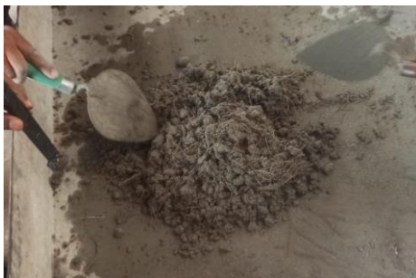
Fig. 5.7 Mixing of Cement mortar with coir
