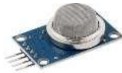
Figure 2 Air Quality sensor
