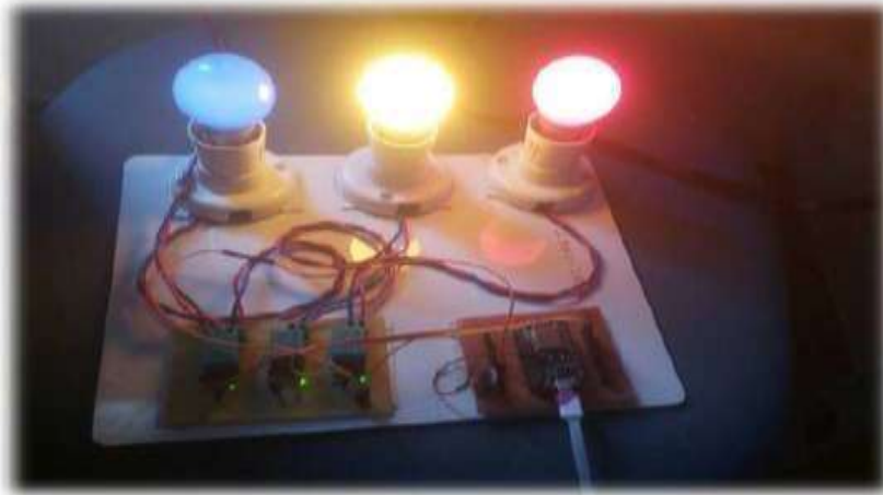
Figure 7. Home appliance control using arduino
