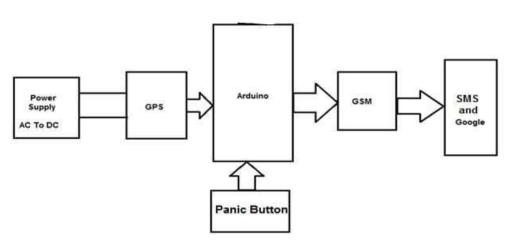
The brain of the system is an AVR microcontroller. The GPS module is connected to the microcontroller via a serial port. The software is connected to the GSM module microcontroller via the serial port.
