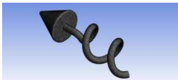
Figure 4: 3D Model of the Meshed Conical Microswimmer.
