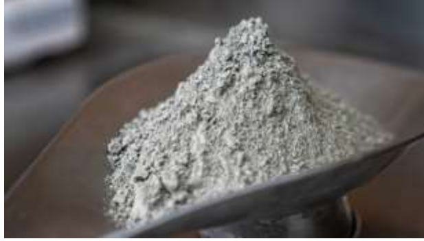
Fig.3.1 Ordinary Portland cement 43 Grade
