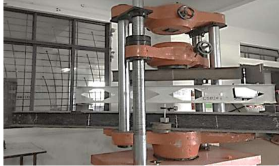
Fig 8 - Testing of Hexagonal 30° Castellated Beam
