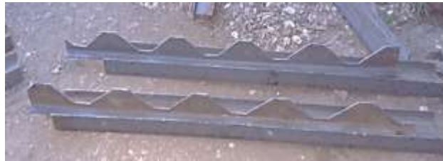
Fig 2 - 30° Hexagonal cutting of castellated beam
