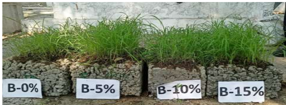
Figure 1 Vegetation concrete blocks with different biochar contents
