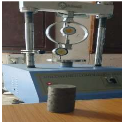
Figure9.1: Unconfined Compressive Strength
