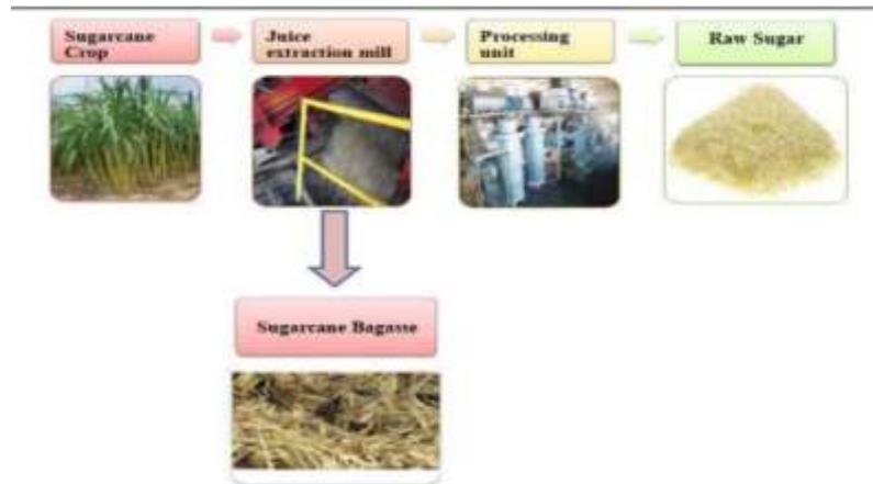
Fig.2.1 Flow diagram for production of raw sugar and sugarcane bagasse
