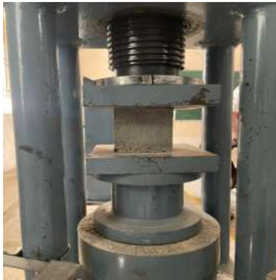
Fig: 4.1.1. Testing of compressive strength
