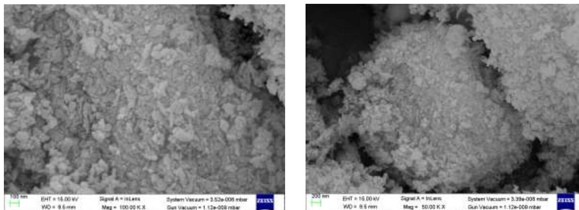
**Figure 3.2:** SEM micrographs of  $\text{SnFe}_2\text{O}_4$  nanocomposites
