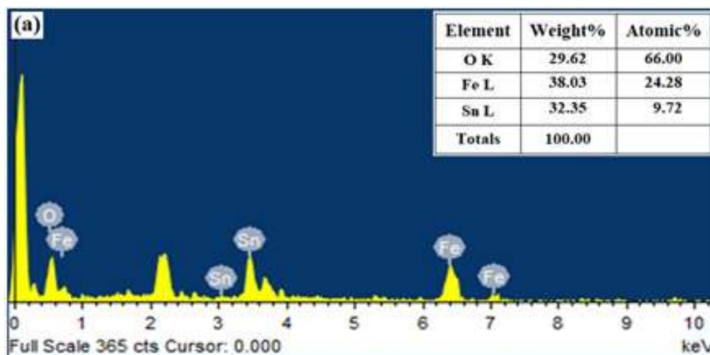
**Figure 3.3:** EDS patterns of  $\text{SnFe}_2\text{O}_4$  nano composite
