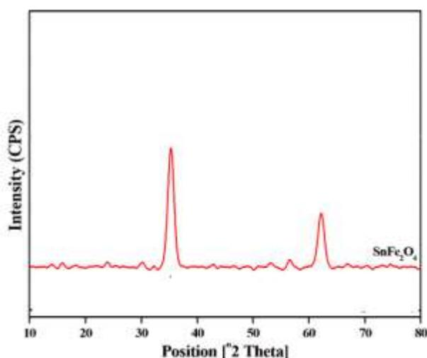
Figure 3.1: XRD patterns of  $\text{SnFe}_2\text{O}_4$  nano composite
