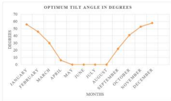
Figure 8.3 Graph on averaged monthly optimum tilt angle on solar panels
