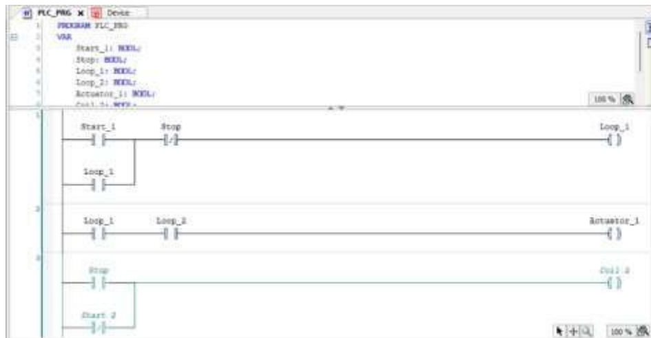
Fig. 1 Ladder Diagram Programming in Codesys
