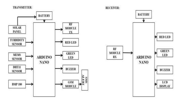
As shown in the block diagram it has 2 boards one is transmitter side and other is receiver side and arduino nano microcontroller is used to process the data. Transmitter side will have solar panel, battery, turbidity sensor and DHT11 sensor, MEMS sensor and BMP 180 sensor in it. The transmitter unit is always present in the sea and it is not possible to constantly charge it time to time, so we use a solar panel to allow it to generate its own power and keep
