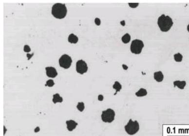
Fig 2 Microstructure of as-cast specimen.
