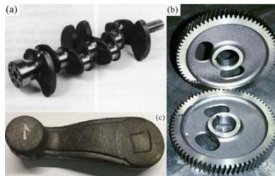
Fig 1 ADI applications (a) ADI crankshaft(b)ADI driving gear(c)ADI pitman arm.
