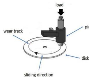
**Fig3 : Pin on Disk Test**
