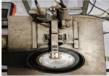
Fig 5 pin-on disc machine.
