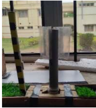
Fig.7. Vertical Axis Wind Turbine of savonius shape
