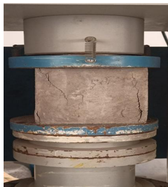
Figure 2: Specimen after Failure for Compressive Strength test
