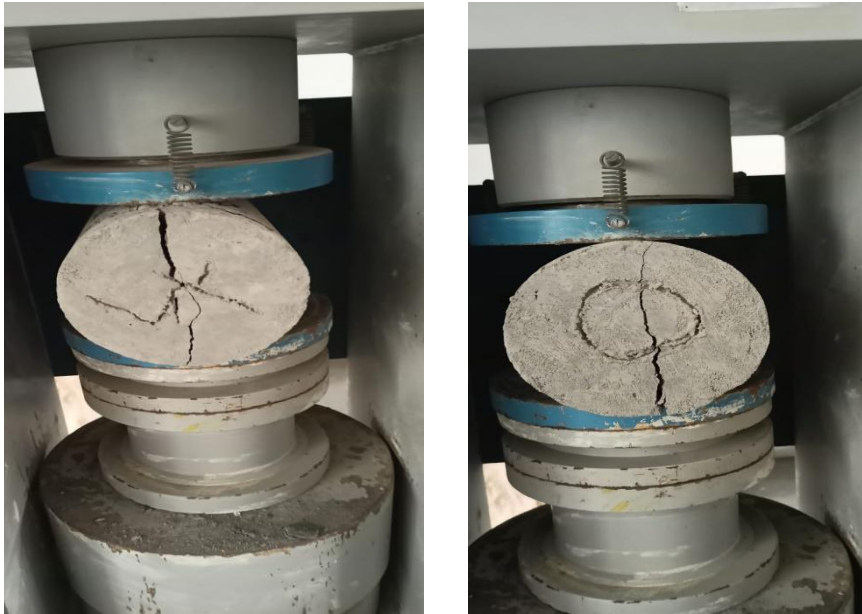
Figure 5: Specimen after Failure for Split Tensile Strength Test
