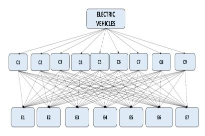
Typically, a pairwise comparison matrix will be 9\*9 cells in size. It is necessary to first generate a pair-wise comparison matrix, then generate a normalised pair-wise comparison matrix.
