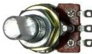
Fig.6. 10K voltage divider
