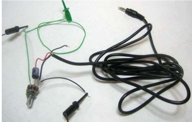
Fig.7. Connection of attenuator circuit with audio cable
