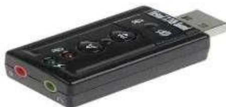
Fig.1. USB sound card is used as the signal input.
