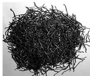
Fig. 2 – Hocked end steel fibers with an aspect ratio equal to 30. (14)
