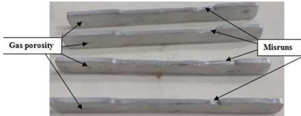
Composite Samples with different defects produced by inclined at 45o pouring of die. [10]
