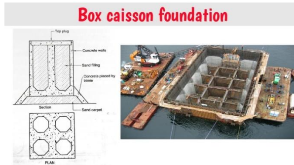
Fig -1 Box Caisson Foundation
