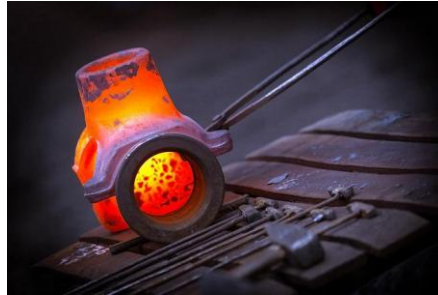
Figure 2 Hot forging process.
