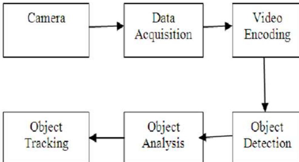
Figure 1 - Block diagram for Intelligent Video Surveillance System
