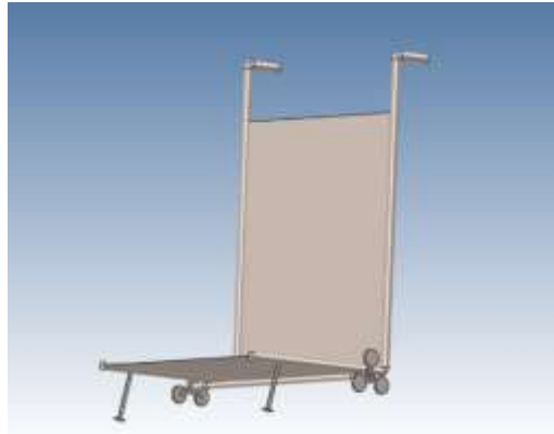
Figure 5: Trolleys final assembly
