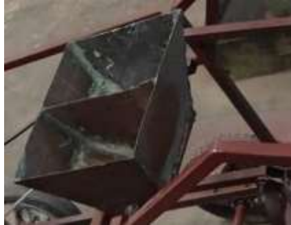
Figure 3 Hopper and seeding
