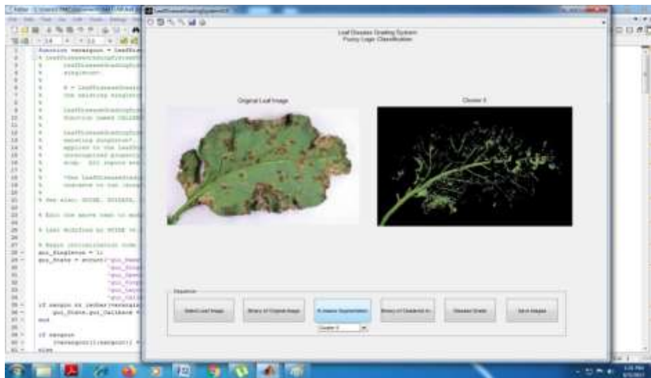
Figure 5: Use K-means to cluster the objects into luminosity layer 'L*' cluster using the Euclidean distance metric
